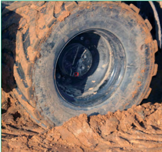
Fig. 16 Truck tire creating rutting on weak subsoil
