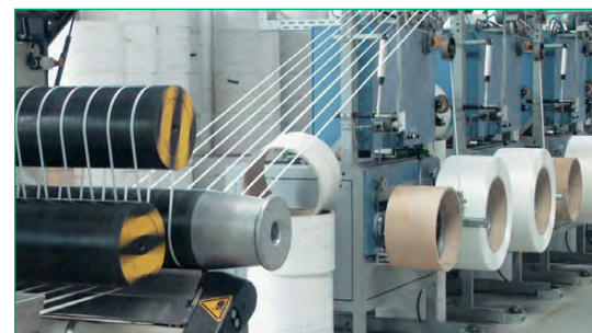
Fig. 4 Stretching process of Secugrid® ribs
