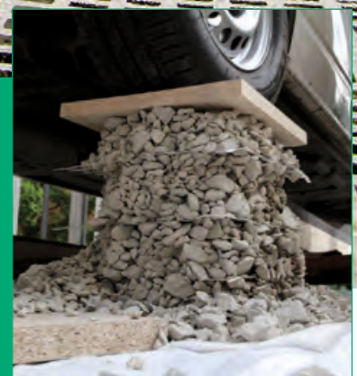
Figure 2 Interlocking effect demonstrated by a Secugrid reinforced gravel column supporting a van (see http://www.naue.com/en/naue-tv/geogrid-experiment.html )
